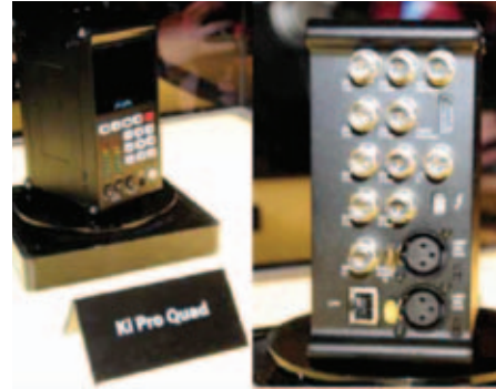
AJA Ki Pro Quad – Removal SSD – Compressed/Uncompressed – Compressed format
