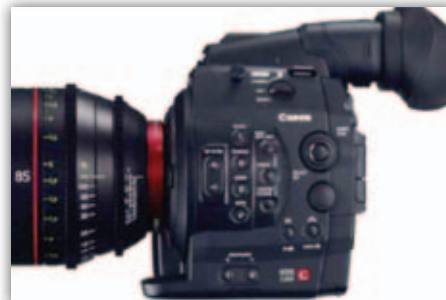
Canon C500 4K Camera – 4K real time output (3G HD-SDI) – AJA Ki pro quad storage – 4K 60P possible
