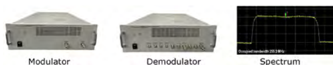
Figure 3-1: Wideband LDM-based modulator and demodulator
