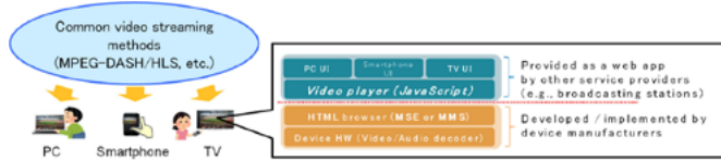
Figure 2-13: Overall structure of a video player that can be used across multiple devices using MSE/MMS
