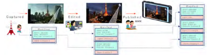
Figure 2-14: Flow of attaching and presenting provenance information
