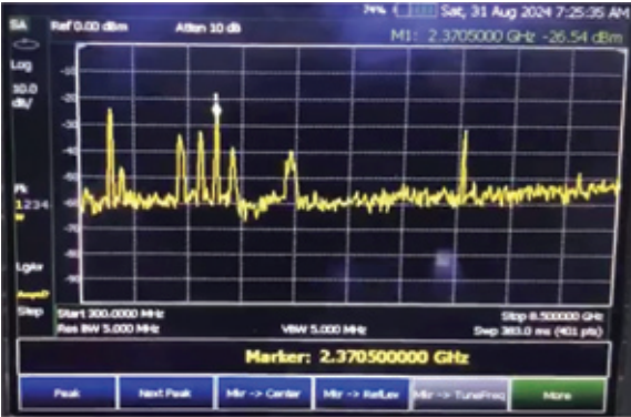
Figure 15: Network Interference Detected Due to Wireless Network Jammer Activation (courtesy of RTM)
