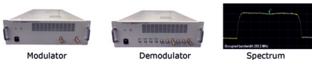
Figure 4-1 Wideband LDM-based modulator and demodulator
